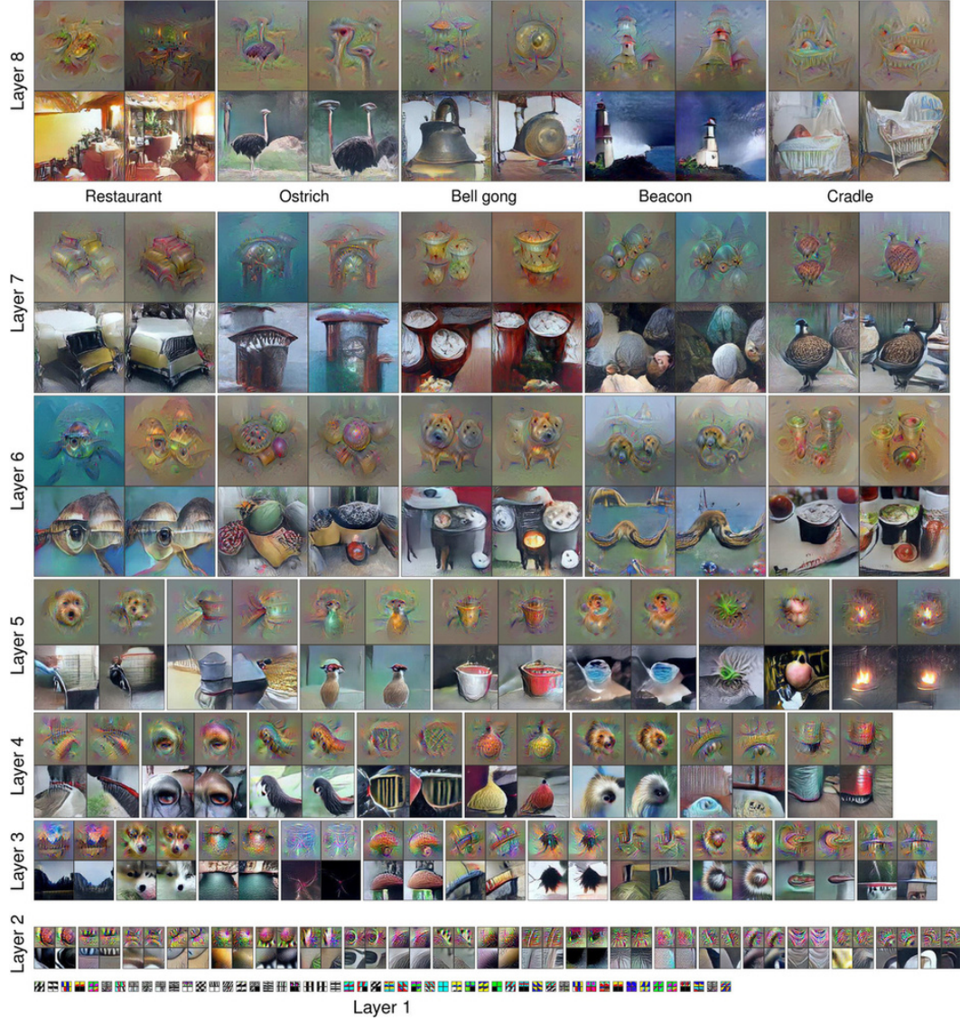
Figure S14: Visualization of example neuron feature detectors from all eight layers of a CaffeNet DNN [24]. The images reflect the true sizes of the receptive fields at different layers. For each neuron, we show 4 different visualizations: the top 2 images are from a previous work that harnesses a hand-designed prior called “mean image initialization” [9]; and the bottom 2 images are from our method. This side-by-side comparison shows that both method often agree on the features that a neuron has learned to detect. In overall, our method produces more realistic-looking color and texture. However, the comparison also suggests that our method does not visualize well animal faces (the 3rd & 4th units on layer 6; 1st unit on layer 5; and 6th unit on layer 4). Best viewed electronically, in color, with zoom.
